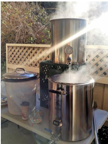
**“The Boil” Transferring fresh wort from the mash tun to the kettle to get the boil started.**
